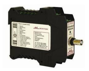
A DIN rail mounted single-sensor signal conditioning unit in a 22.5mm format providing early warning of bearing and gear faults, imbalance, misalignment and looseness. Three different vibration output signals; AC acceleration for vibration analysis with on-line or hand-held FFT data collectors, velocity for overall machine vibration and peak acceleration for bearing wear for continuous monitoring in industrial controllers, PLCs etc. in either analogue or digital format.
