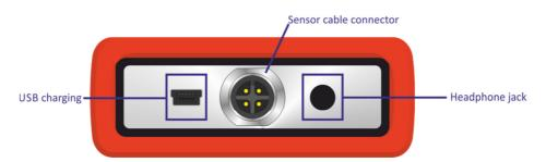
The headphone jack will accept a 3.5mm stereo jack plug. Headphones (not included) may be used to listen to the vibration directly. A datalogger can also be connected to the headphone jack.
