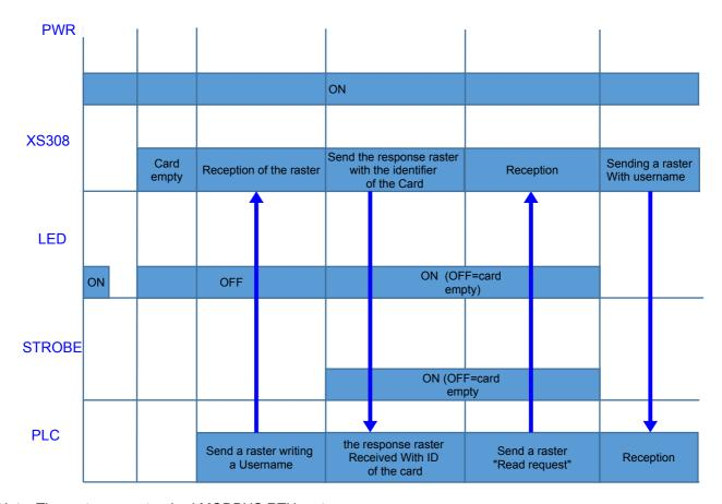
Note: The rasters are standard MODBUS RTU rasters.
